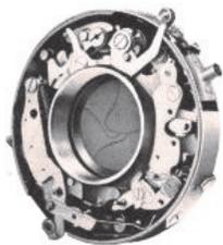
The five blade action of the shutter of PETRI 1.9 gives you accurate readings from 1 to 1/500 second, and includes a bulb setting. The shutter also has a built-in self-timer and is equipped with M.X.S. synchronization which is adaptable to all kinds of flash bulbs and electronic flash.
